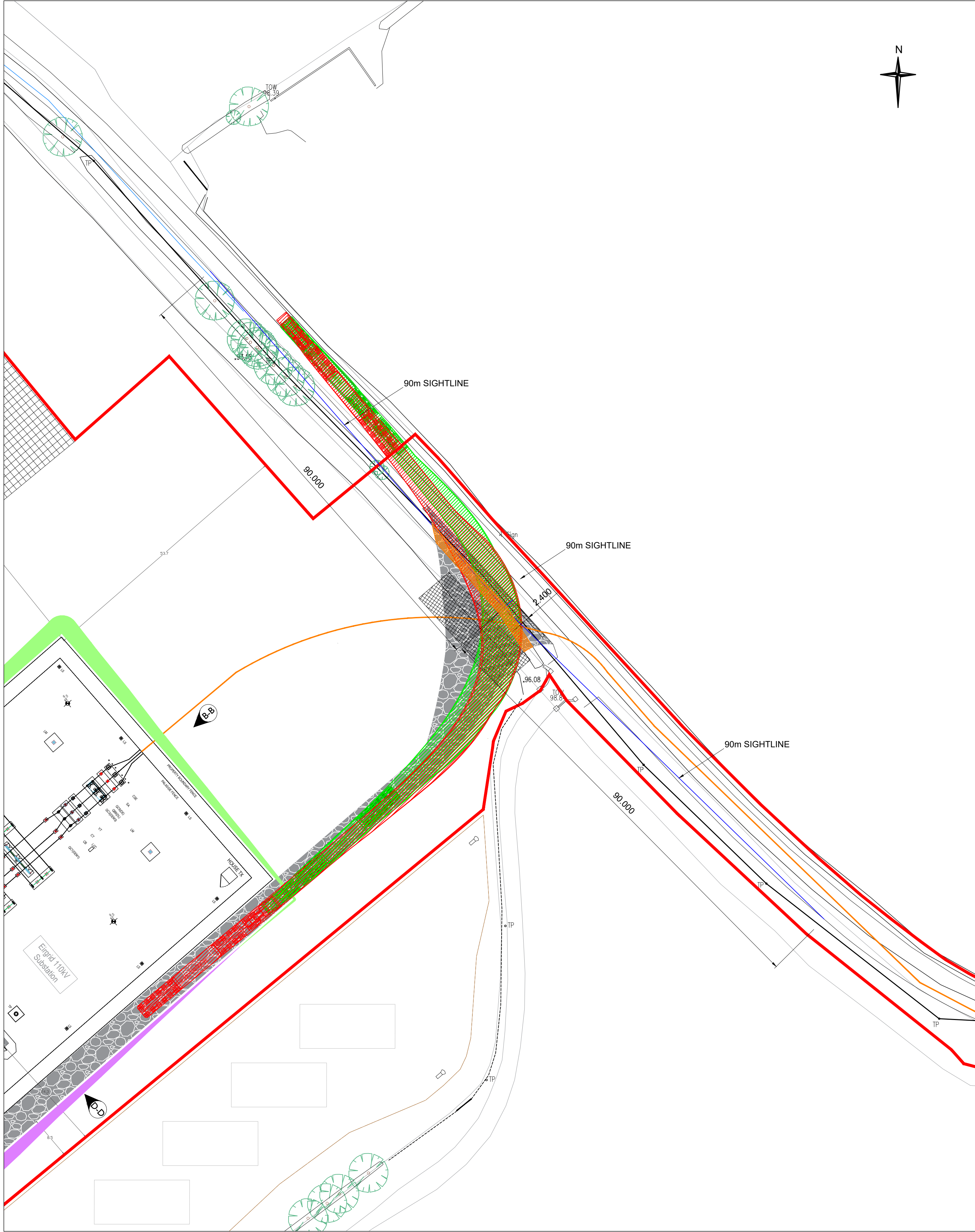
PROPOSED SITE ACCESS 1 - SIGHTLINES (Scale 1 : 500)
